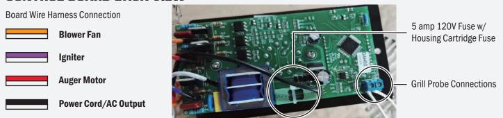
The circuit board is equipped with a 5 amp, 120V fuse to help protect against power surges and electrical shorts. When not in use, always unplug and store your grill. This will help prevent electrical damage from power surges or storms.
