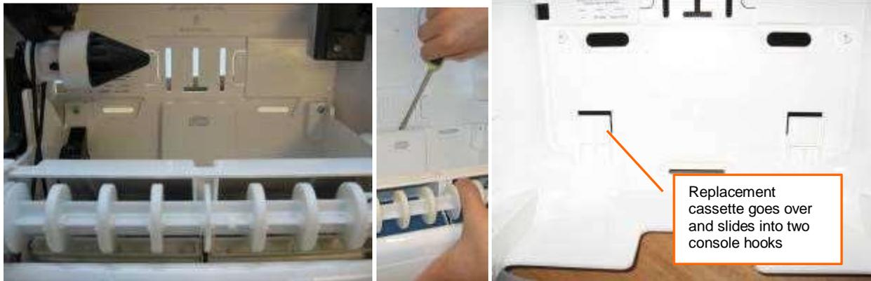
1. Remove two Phillips head screws holding the cassette to the console.
