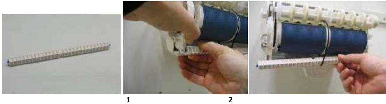
1. Bend out the fitting hole on the left side.
