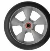
Microcellular Foam - 10 in - 111075 10 x 2.75 inch puncture resistant, non-marking microcellular tire with one-piece high-density, interlocking polyethylene hub with semi-precision... bearings
