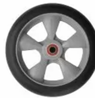
Microcellular Foam - 10 in - 111070 10 x 2 inch puncture resistant, non-marking microcellular tire with one-piece high-density, interlocking polyethylene hub with semi-precision.. bearings
