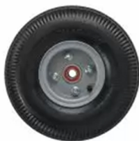
4-Ply Pneumatic - 10 in - 121060 10 x 3.5 inch tube-type tire with three-piece off-set hub and semi-precision bearings
