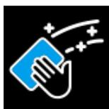
**Cleaning and switch off.** This is a special function to rapidly cool the oven down to 122 °F (in around 10 minutes if the user opens the door), after which the oven automatically turns itself off.
