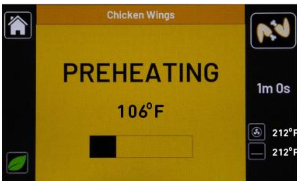
When the set oven temperature is reached the oven will beep, the screen will go green and the oven is ready to be loaded with product.
