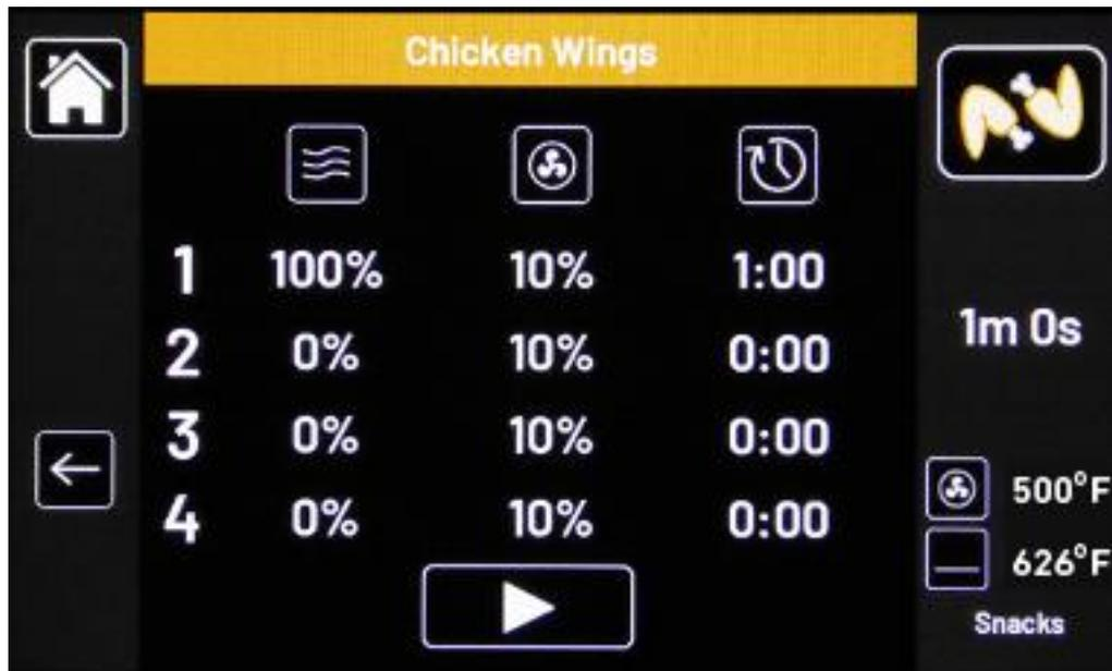
The Recipe editing screen consists of 4 rows of cooking stages (not all will need to be used for most recipes), with 3 columns to set Microwave Power, Fan Speed and Time.
