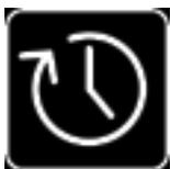
**Time.** This is seconds and minutes based and can be adjusted in 5 second intervals from 0 seconds to 30 minutes
