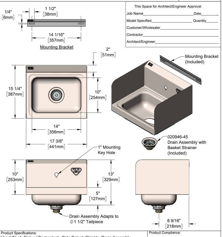
Hand Wash Sink w/ Backsplash, Side Splash Shields, Drain Assembly and Mounting Bracket, NSF Approved, Stainless Steel, 17" x 15" Overall, 14" x 10" Bowl, Single Faucet Mounting Hole, 3 1/2" Drain Hole
