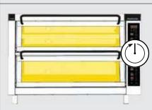
**4.** When the oven reaches 300 C (which takes about 20 minutes), leave it switched on for 1 hour.
