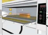
3. Clean Stone Brush and scrape out bake deposit or soot regularly during the day. Use a metal and soft brush!
