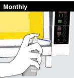
7. Lubricate Lubricate all the door bushings.
