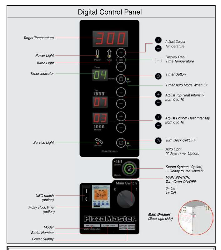
Power: A yellow lamp indicates that the heating element is on.
