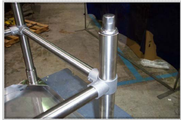
Figure 2—Cross brace set-up
