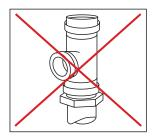
The dishwasher flexible drain hose must be connected to a WYE fitting.
