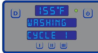
7. After the wash cycle is complete, the machine will automatically enter the rinse cycle.
