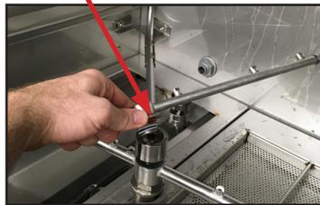
5. Verify the nozzles and arms are free from obstruction. If clogged, remove end-caps, clean nozzles with a brush, and flush with fresh water.
