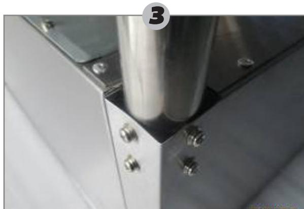
Install legs **(D)** into gussets using screws **(I)**. Make sure the rivet in leg is closer to gusset than to foot end.
