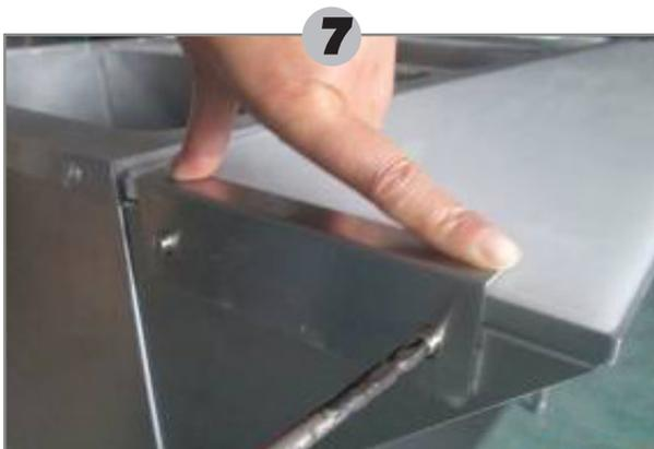
Using screws (#I) fix the end brackets (#H) on the shelf supports (#F) and tighten to secure the poly board on the front shelf.
