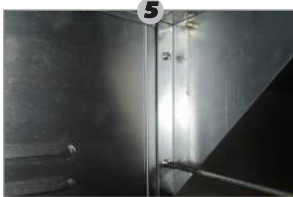
Using screws (#G) to fix the front shelf supports (#F) on the base (#A).
