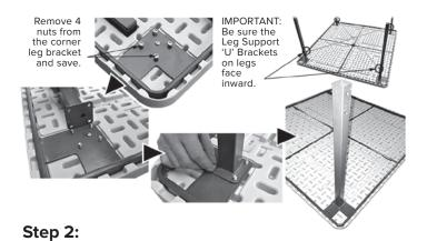
Unscrew the nuts from the corner bracket under the Table top. Position a table leg onto these bolts and secure by using those four nuts. Make sure that the welded 'U' Bracket faces the center of the table
