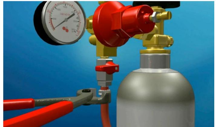
**Attach the red pressure tubing to the gas regulator.**
