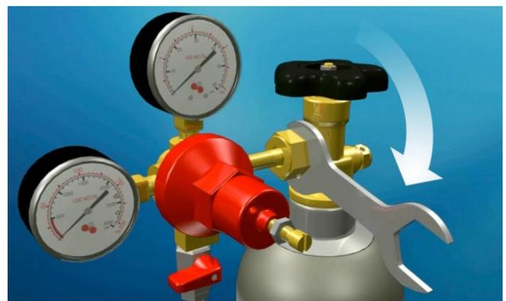
Tighten the tank nut.
