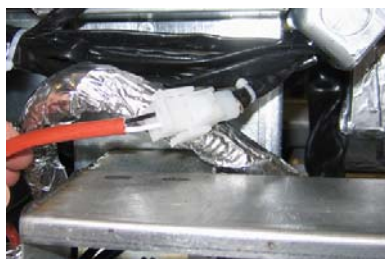
Figure 6: Attach the two-pin white connectors and plug the black connector into the utility box as shown. * Note the position of the black connection may differ from photo.
