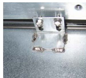
Figure 5: Attach the melting unit to the rails on both sides.
