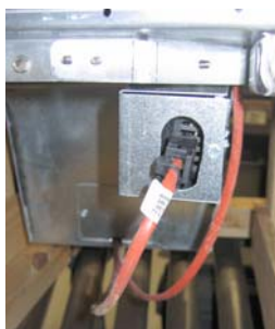
Figure 6: Attach the two-pin white connectors and plug the black connector into the utility box as shown. * Note the position of the black connection may differ from photo.
