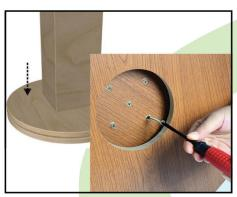
Fix the square wood pipe on the bottom. Use 1.5" screws (x5)
