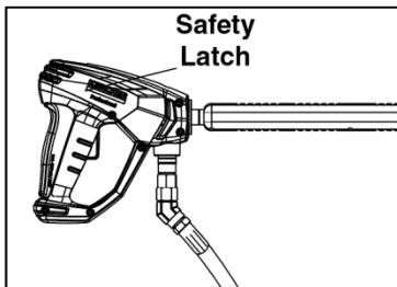
**STEP 5:** Engage the spray gun safety lock.
