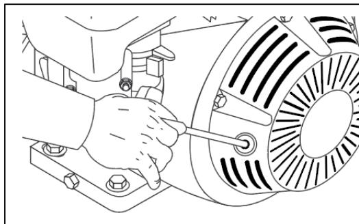
**STEP 9:** Pull the starter grip. If the engine fails to start after 2 pulls, squeeze the trigger gun to release pressure and repeat step. Return starter cord gently. After the engine warms up enough to run smoothly, move choke to run position and throttle to fast position.
