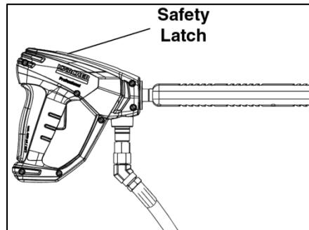
**⚠ WARNING!** Never replace nozzles without engaging the safety latch on the spray gun trigger.
