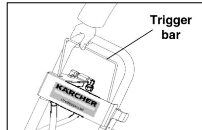
**STEP 6:** Pull trigger bar to drain water from surface cleaner swivel and spray arm.
