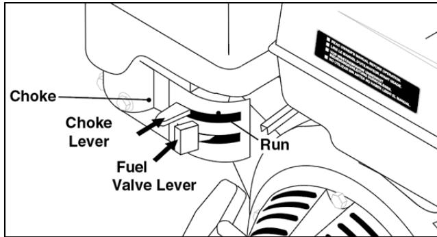
**STEP 7:** Move the choke lever to the "Choke" position (on a warm engine, leave the choke lever in the run position).
