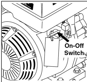
**STEP 8:** Turn the engine switch to "On" position.
