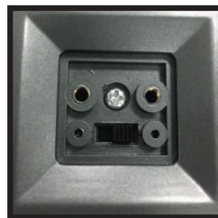
The calibration switch is located underneath the scale base. When the switch is set towards the USB or RS232 interface, it means CAL switch is on. When the switch is set towards the power switch, it means the CAL switch is off.
