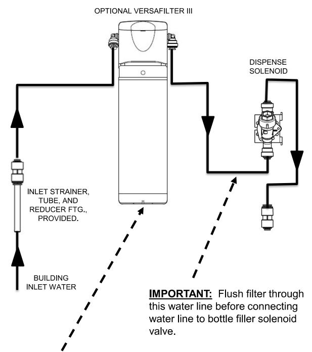
**IMPORTANT:** When replacing filter cartridge, depressurize water lines prior removal of filter housing from the quarter turn filter head assembly.
