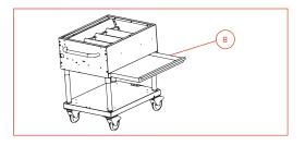
Insert the grease tray(s)(8) into the back of the grill.
