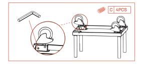
Fasten legs (3) to the base using Allen wrench (A) and Screw-C (4PCS).
