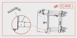
Tighten the legs (3) to the grill body section (5) using the Allen wrench (A) and Screw-C (4PCS).
