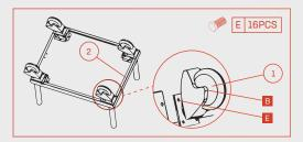
Install casters (1) to under shelf (2) using Bolt-E (16PCS) and Spacer-B (16PCS).
