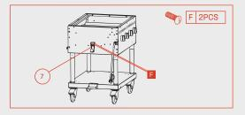
Attach the top propane tank holder (7) to the grill body section (5) using Screw-F(2PCS).
