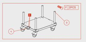
Install propane tank holder (4) to the under shelf (2) using Screw-F (2PCS).
