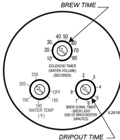
Fig. 15 Adjust Brew Time and Dripout Time
