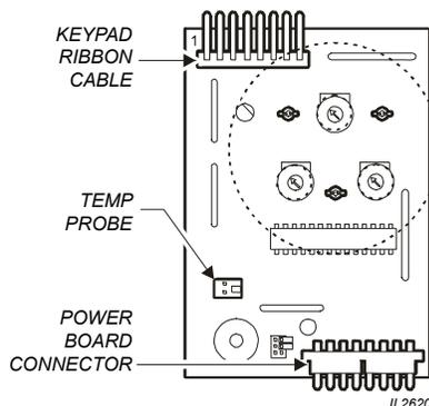
Fig. 18 Controller Hook-Up
