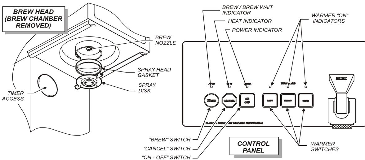
Fig. 1 Features & Operating Controls
