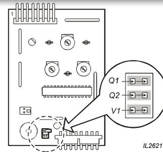
Fig. 19 Controller Jumpers
