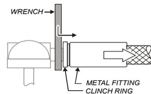
SLIDE WRENCH BETWEEN VALVE AND HOSE FITTING
