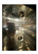
3. Notice if there is any residue of the gasket material remaining around the light fixture or on the light globe itself. If so, remove it with a soft cloth.
