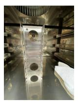
6. Place the Pan-stop/Light Guard over the light fixtures allowing the screws of the top light fixture to sit on the corresponding holes of the Pan-stop/Light Guard.
