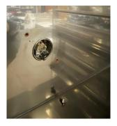
5. Remove the plastic material from the Pan-stop/Light Guard.
