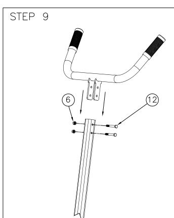
Slide handle onto post and fasten with two locknuts(6) and two bolts(12).
