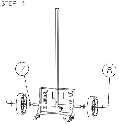
Secure wheels using four washers(7) and two cotter pins(8).
