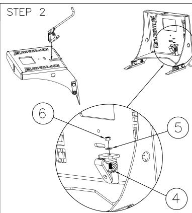
Insert kickstand through rear of base and secure using one bolt(4), one washer(5), and one nut(6).
