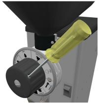
(7) Replace right screw on knob. (8) Replace left screw on knob.
