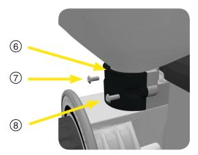
Replace the outer hopper collar, then the two screws.
