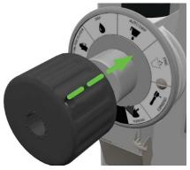
(6) If the decal is placed in the correct location (the screws should both show through the decal), then press to adhere. Now, replace knob.
