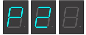
3. Press and release the upper hidden button once more. The display will show **P2**. Display will now show the “SET” temperature (ex: 200). Press the (+) button to increase the temperature set point, or the (-) button to decrease the set point.
