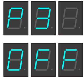
5. Press and release the hidden button once more. The display will read **P4**. This will toggle the energy save mode from 60°C (140°F) or tank heater “OFF”.
