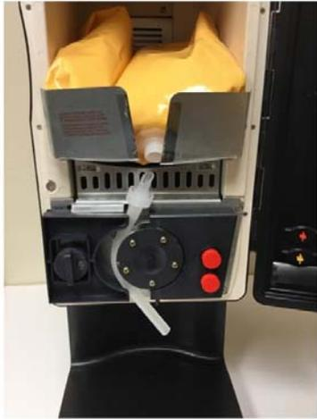
**Step 5.** Open dispenser door and remove upper warming tray. Place pouch in lower oven tray with the spout and tube directed toward the front of the machine and downward through the opened tube clamp (rotate cam counterclockwise to open).
