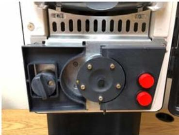
**Step 4.** Open the front door of the warming dispenser. Open the tube clamp by turning the cam counterclockwise.
