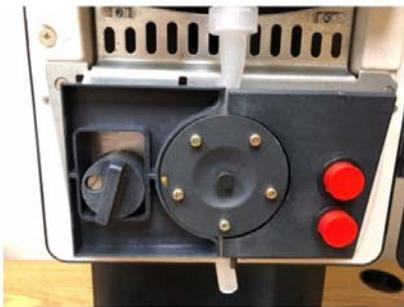
**Step 7.** Close the tube clamp by turning the cam clockwise; locking it in place. If desired, place unopened reserve pouch in upper warming tray to preheat. Close the warming dispenser door.
