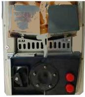
Step 5. Open dispenser door and remove upper warming tray. Place pouch in lower oven tray with the spout and tube directed toward the front of the machine and downward through the opened tube clamp (rotate cam counterclockwise to open).
