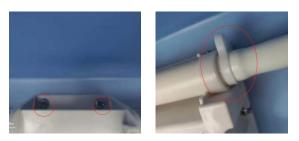
6. Disassemble fixed screws which are in the spray pipe. Dismantle the spray pipe.
