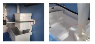
5. Remove screws which are securing the spray pipe. Remove the spray pipe and the upper pipe.
