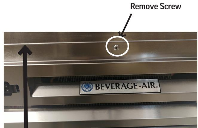
Push Panel Up to Release From Screw Heads Behind Panel
