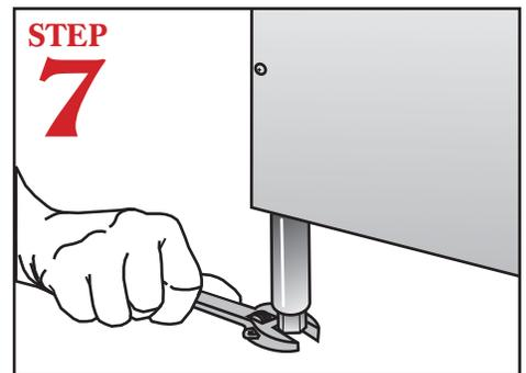
Level dishwasher by adjusting leveling legs. Dishmachine must be level front and back.
