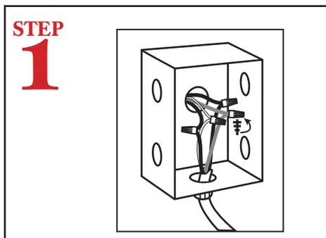
Connect hard wire power supply from dishmachine to power box. (Two hot wires, one neutral and one ground.)
