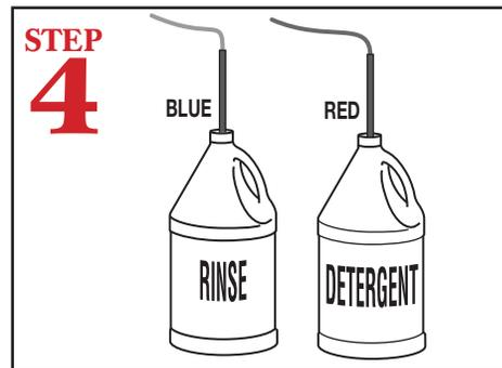
Insert tube stiffener with chemical tubing into corresponding chemical dispensers.
