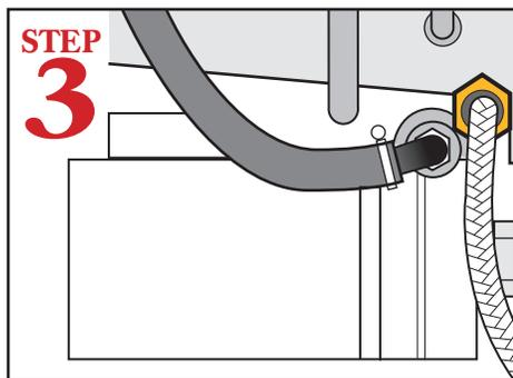
Connect dishmachine to hot water source 120°F - 140°F. Minimum temperature will remain in wash cycle until booster heater temperature reaches 180°F, then it will advance into rinse cycle.
