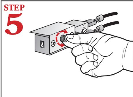
If necessary adjust the temperature by turning the adjustment stem clockwise to increase.
