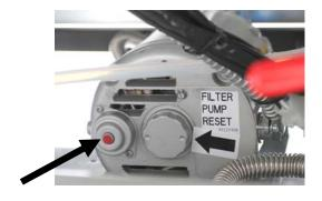
Filter Pump Reset Switch
