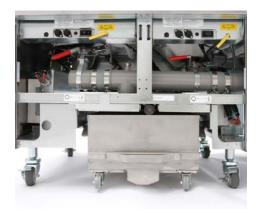
The filter pan slides under the fryer (left), connecting with a male connector (right). Ensure that the pickup tube is securely coupled with this connector. Its location may vary based on model.
