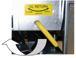
Allow the oil to bubble for 10-15 seconds to ensure evacuation of all oil in the return lines and turn the yellow handle to left to deactivate pump.
