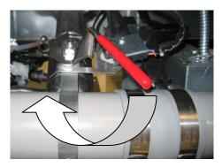
After filtering is complete, push the red drain handle (left) to close the drain and start refilling the frypot.
