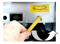
Turn the yellow handle (right) to open the oil return valve and activate the filter pump.
