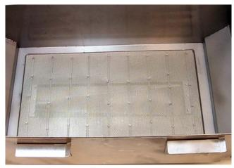
Support grid properly placed in filter pan.
