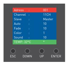
ESC Is used to navigate to the previeous higher-level menu item.
