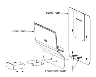
Remove Front-Plate from Back-Plate by pulling the Front-Plate off the threaded studs.
