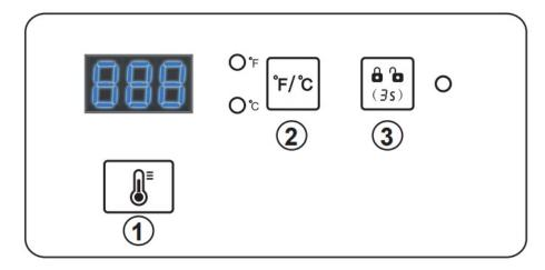
There are 3 LED blue lights: °F, °C and lock. When the unit is plugged in, all lights will be on for 1 second. There are 3 buttons: temperature setting °F/°C switch and lock.
