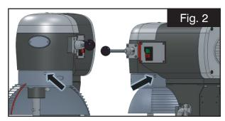
Remove the rubber closing caps from the mounting screws at noted locations. Then remove the screws. (Fig. 2)
