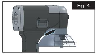
4. Remove the cap and mounting screw at noted location. (Fig. 4)
