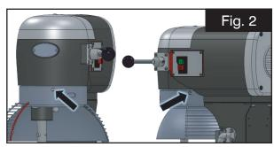
2. Remove the rubber closing caps from the mounting screws at noted locations. Then remove the screws. (Fig. 2)
