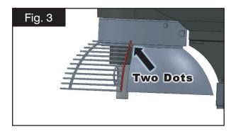
3. Turn the wire guard until the edge of the wire aligns with the two indentation markers on the fixed rear guard. (Fig. 3)
