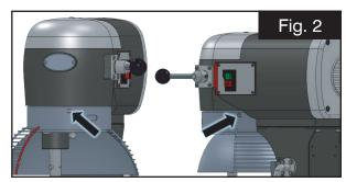
Remove the rubber closing caps from the mounting screws at noted locations. Then remove the screws. (Fig. 2)
