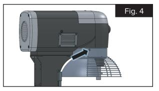
4. Remove the cap and mounting screw at noted location. (Fig. 4)
