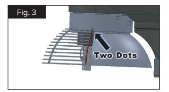
3. Turn the wire guard until the edge of the wire aligns with the two indentation markers on the fixed rear guard. (Fig. 3)
