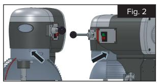
2. Remove the rubber closing caps from the mounting screws at noted locations. Then remove the screws. (Fig. 2)
