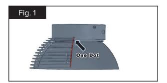
1. To remove the wire guard, adjust the position to align the edge of the wire guard with the single indentation marker on the fixed rear guard. (Fig. 1)
