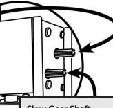
Slow Gear Shaft With the Handle attached, turn counterclockwise to raise the Plunger; clockwise to lower the Plunger
