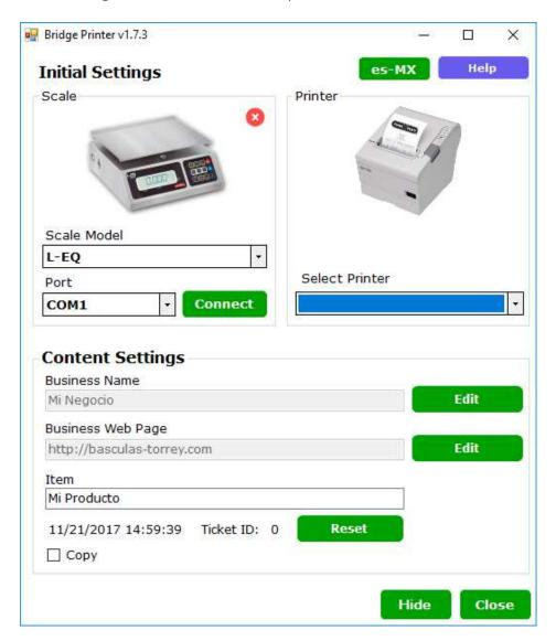
3. Select your scale model using the "Scale Model" drop-down list:
