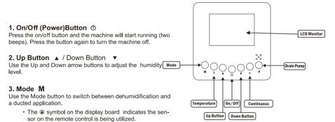
• The • symbol on the display board indicates the sensor on the dehumidifier is being utilized.
