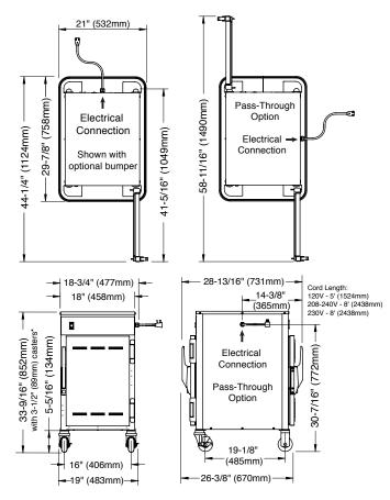
\*31-7/8" (809mm) - with optional 2-1/2" (64mm) casters \*35-1/4" (895mm) - with optional 5" (127mm) casters \*33-15/16" (861mm) - with optional 6" (152mm) legs
