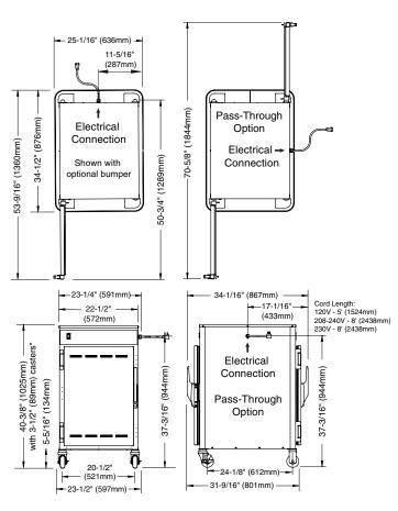
\*38-11/16" (982mm) - with optional 2-1/2" (64mm) casters \*42-1/16" (1068mm) - with optional 5" (127mm) casters \*40-3/4" (1034mm) - with optional 6" (152mm) legs
