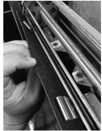
Figure 6. Connecting Belt Wrap Hooks
