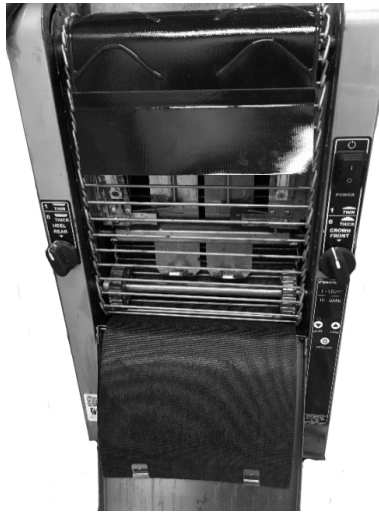
Figure 5. Replacing Belt Wraps
