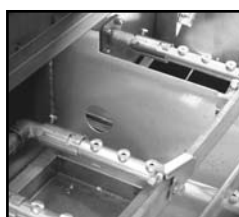
3-stage washing process provides pre-wash, power wash and final rinse all in a 44" machine.
