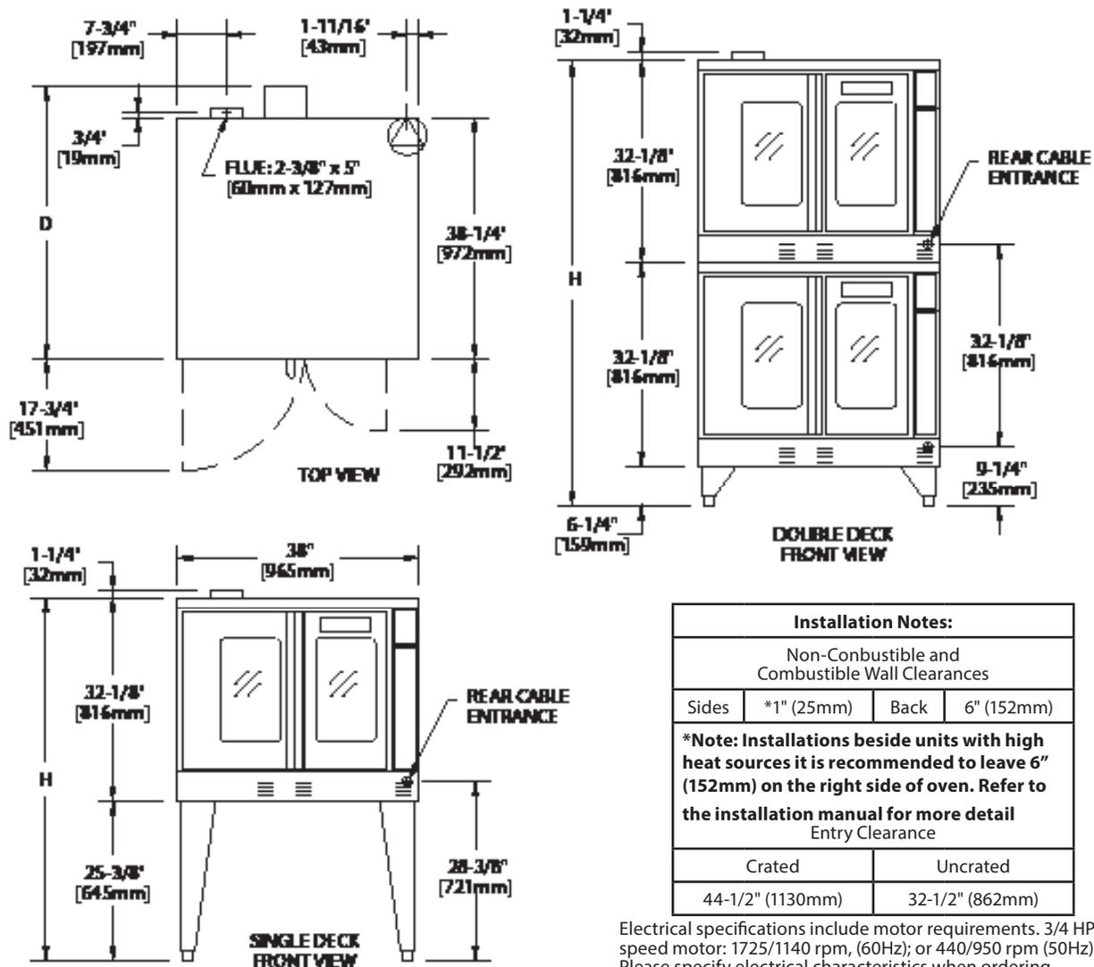
Electrical specifications include motor requirements. 3/4 HP, 2 speed motor: 1725/1140 rpm, (60Hz); or 440/950 rpm (50Hz). Please specify electrical characteristics when ordering Form# MCO-ES/ED-10/20 (04/14/15)
