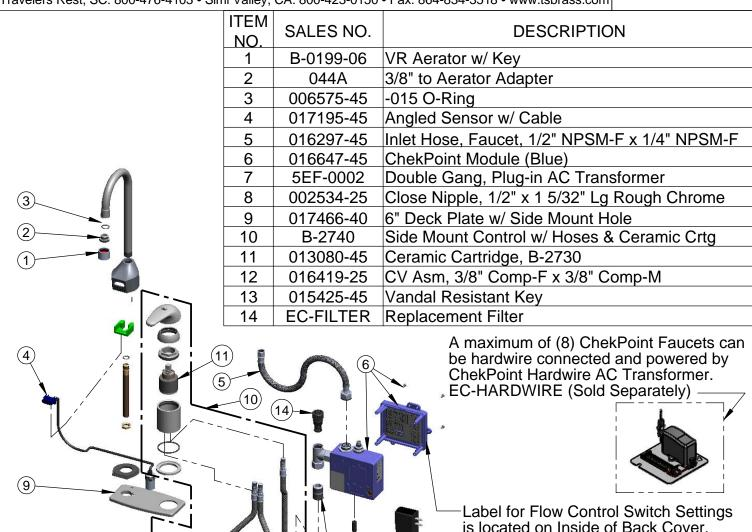
Flow Control Switches are located inside Module Housing in Black Box next to Battery Compartment. \*Switches are set to DEFAULT position: Auto Time Out = 10 seconds Shut Off Delay = 1 second Auto Flush = OFF
