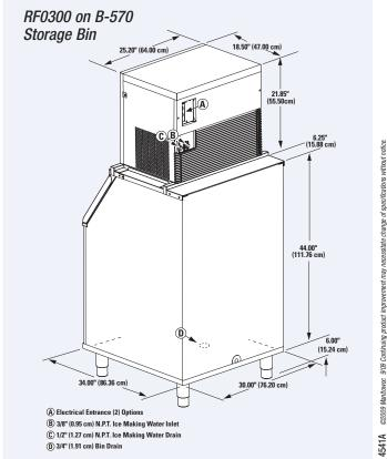
**Installation Note -** Minimum installation clearance: Top/sides: 8" (20.32 cm), back: 5" (12.70 cm).
