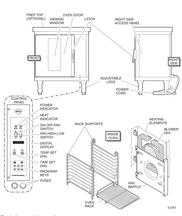
Fig. 1 Features & Operating Controls
