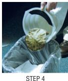
When tea no longer drips from the funnel tip, carefully remove the brew funnel and discard the used tea pouch. Return the power switch to OFF to prevent a false start. Thoroughly clean and sanitize the brew funnel and funnel tip screen.
