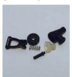
Turn the faucet in a counterclockwise direction and remove the faucet from the dispenser. Unscrew the faucet cap from the faucet body and disassemble all faucet parts.
