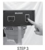
Slide the loaded brew funnel into the funnel rails until it stops. Place the power switch in the ON position. Momentarily press and release the START switch.
