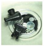
STEP 4 Allow the parts to soak in a sanitizer solution for a minimum of ten minutes.
