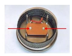
Step 5 – remove slinger plate by loosening the 2 nylon acorn nuts.
