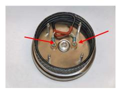
Step 6 – disconnect the two heater lead terminations by removing 2 nuts..
