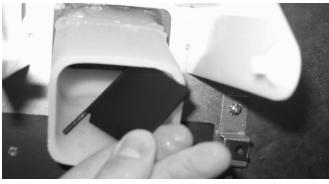
7. Pull the paddle wheel guard from the holes inside the ice dispense snout.
