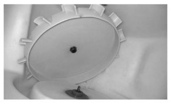
4. Slide the paddle wheel from the motor shaft and remove.
