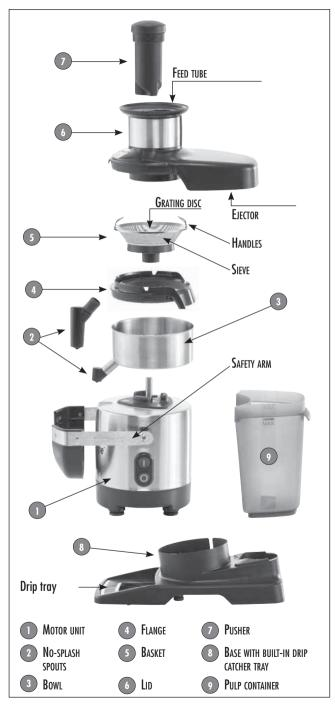
1) Place the motor unit on its base so that the On/ Off buttons are facing you. Pass the power cord through the slot provided.
